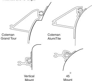
Attach the appropriate bracket to the end of the rafter with the angled cut of the rafter facing the awning rail. Use the #8 pan head screw with the #8 nut, nylon insert, and be sure to place the rafter bumper on the end as shown.
