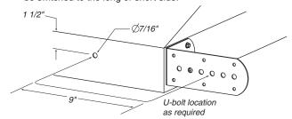
C. When the frame is offset, the back of the coupler should be in line with the side wall. From the side wall the U-bolt should stick out 3-1/4".
