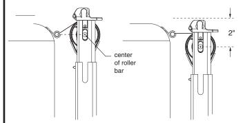
The awning is set from the factory at the lowest position and should be adjusted as required.
