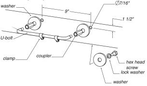
If the frame is offset from the side of the of the camper wall at any distance, then the 5" long threaded stud will be used as follows:
