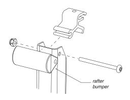
B. For the vertical mount and 45° mount brackets only, slide the rafter and top bracket onto the end of the awning rail and centered behind the arm. Secure the bracket with a #8 self-drilling screw through the top of the bracket and through the awning rail.
