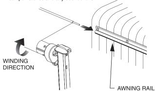
D. Remove the strapping tape from the around the travel lock on the front end of the roll bar. And for Super Sports 10' and over, remove the lock pin from the side of the arm.
