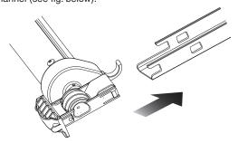
E. WITHOUT REMOVING THE STRAPPING TAPE FROM THE BRAKE LEVER, repeat step 2D using the locking end of the roll bar with the front arm.
