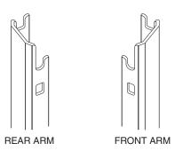
The rear arm has a slot for the roller bar shaft facing the front.
