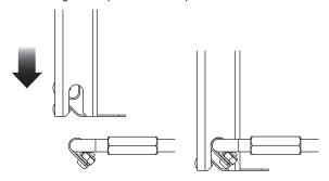
B. Adjust the collapsed height of the arms using the stop bolt located at the bottom and rear facing side of each arm. The roll bar center line should be in line or slightly above or below the awning rail center line (see fig. below).
